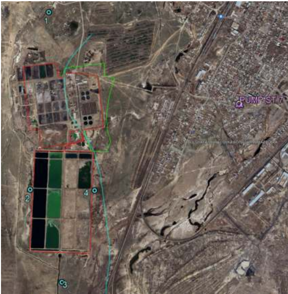
Figure 6.23 Location of sources of groundwater data: Pump station 7 and groundwater monitoring wells (1-4) adjacent to the existing WWTP.
