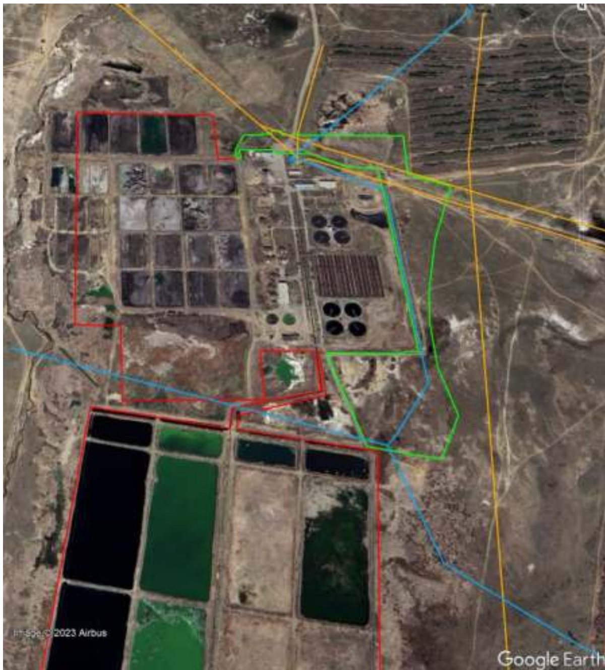
Figure 3.8 Existing overhead powerlines and proposed plot for the new WWTP (Blue: 35 kV overhead powerline. Orange: 6 kV Overhead powerline).
