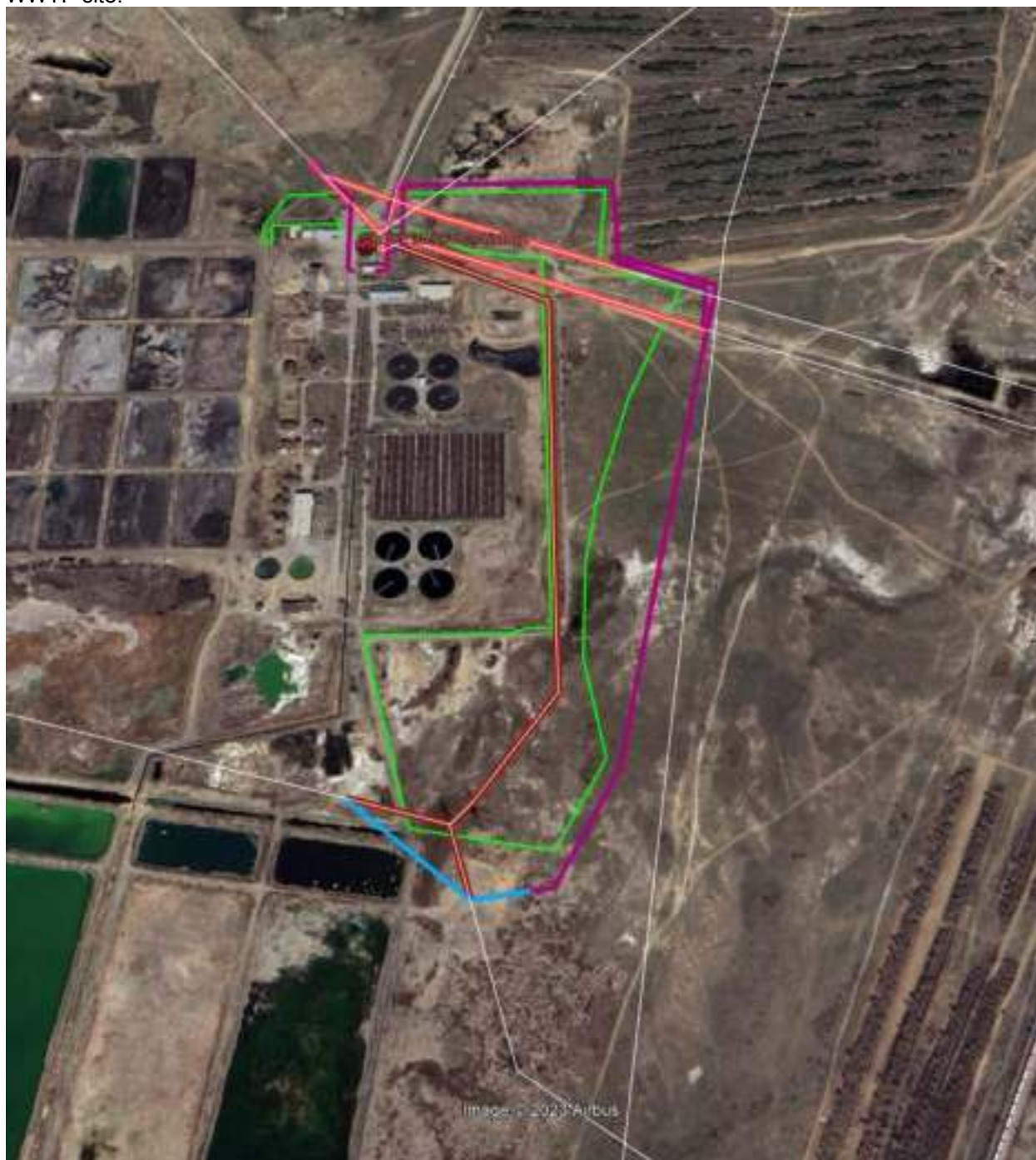
Figure 3.9 Proposed new underground cables (purple lines) and existing overhead power lines which will be removed (dark red over white: 35 kV OHL, light red on white: 6kV overhead lines) and replaced by either underground cables (purple) or a short section of a 35 kV overhead line (blue line) at the south of the site.
