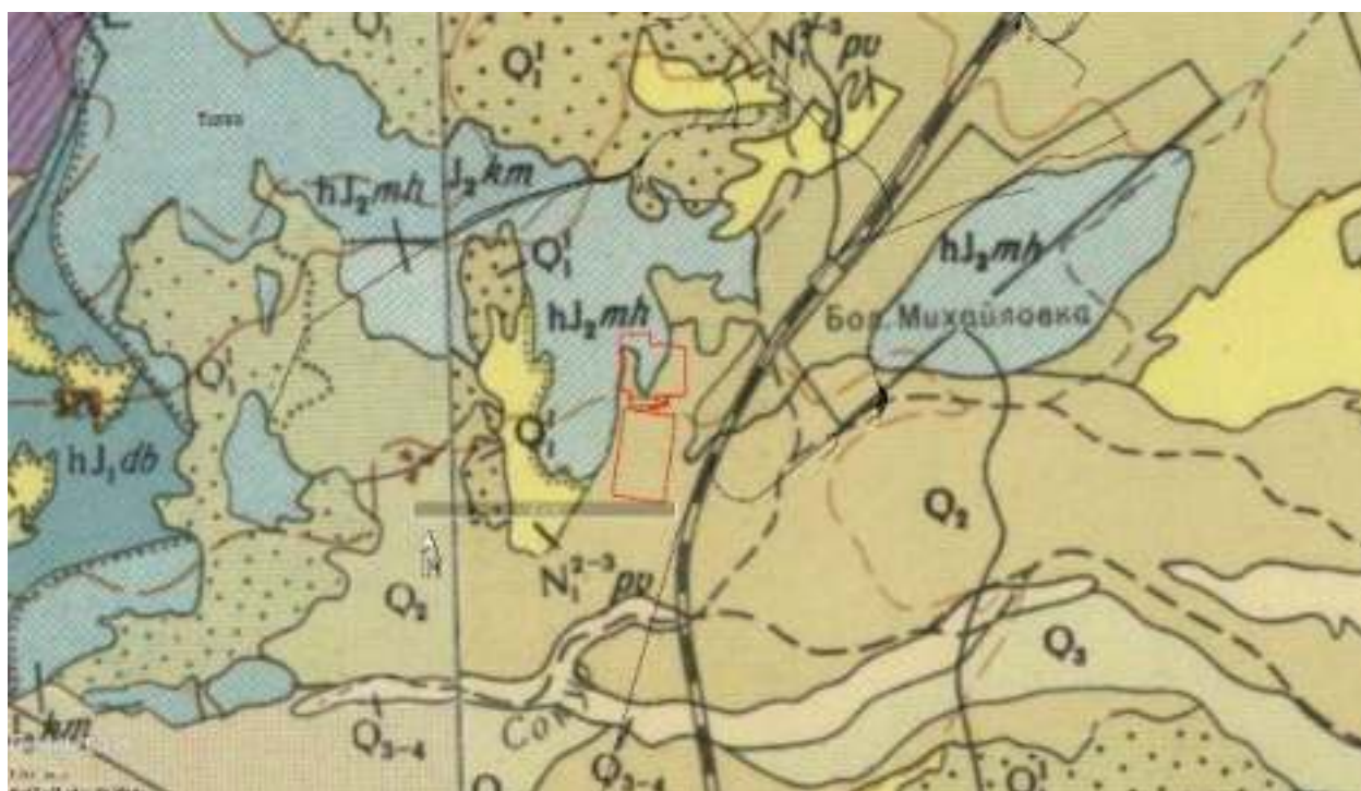
Figure 6.6 Geological map of the WWTP area and surroundings showing that Neogene clay that protects deep groundwater (from the seepages is absent at the sludge beds area (from https://gis.geology.gov.kz/portal/apps/webappviewer/index.html?id=ef1f588363844f7cb1f646e05558da32 ).
