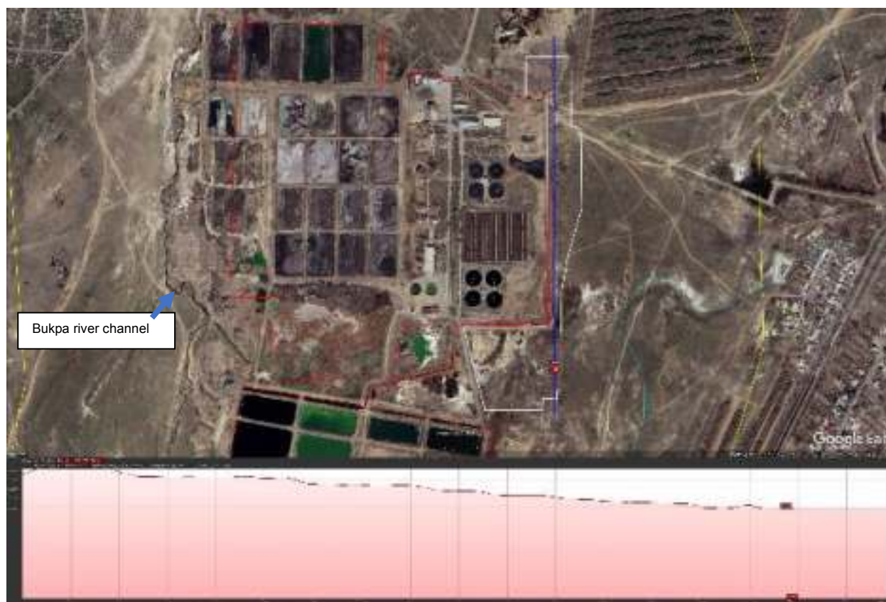
Figure 6.5 Elevation profile (blue line) through the new WWTP site from N to S (blue line and corresponding transect from up left to right, respectively). The white line to the east of the existing WWTP indicates the boundaries of the site extension required for the proposed new WWTP.
