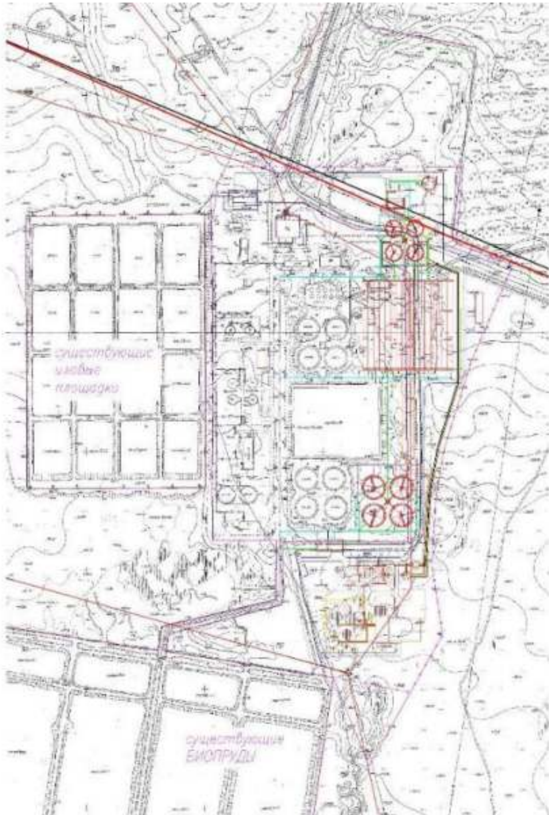
Figure 6.2: 1:2000 topographic map of the existing and projected WWTP site (Source: Aquarem, 2023 ) Existing 110 and 35kV powerlines are shown in red. Planned redirection of the powerlines are shown in purple.
